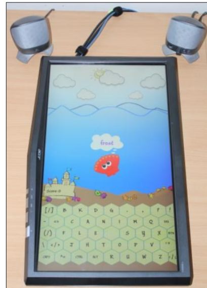
Figure 1. The apparatus used in the experiment. Each target word appeared in a speech bubble in the center of the screen. Participants drew the corresponding gesture on the ATOMIK keyboard located at the bottom of the screen.
