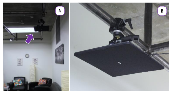
Figure 6. The (a) Voices in My Head concept uses (b) directional speakers to selectively provide information.
