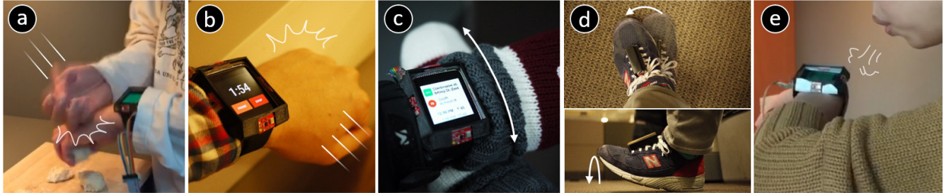
Figure 1: Examples of no-handed smartwatch interaction techniques: (a) Slap, (b) Bang, (c) Swipe, (d) Foot Tap, and (e) Blow.
