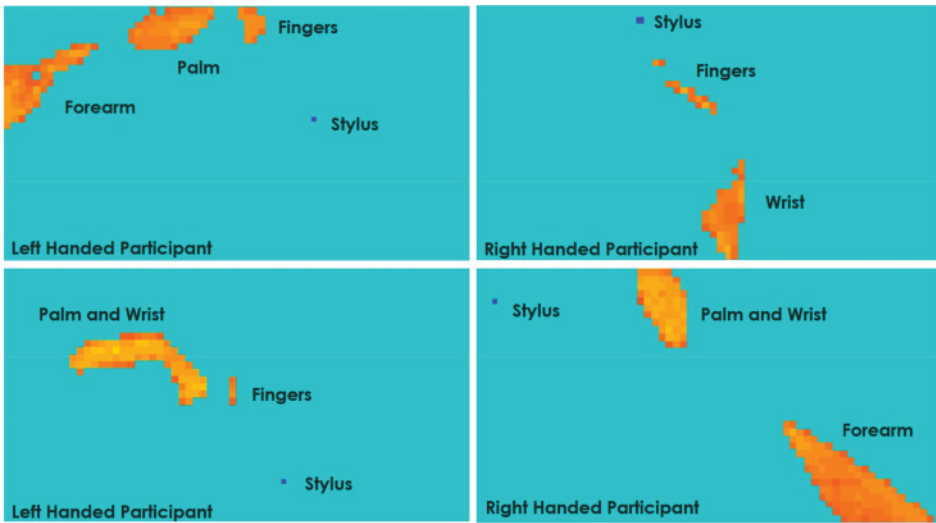
Fig. 2. Example data provided by pen and touch digitizers. The stylus location is represented in dark blue and the touch data is represented in orange, with the darker shades representing the higher levels of activation. All touch data in these images is unintended and should not be accepted.
